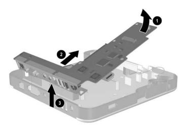
Removing the Board Assembly
